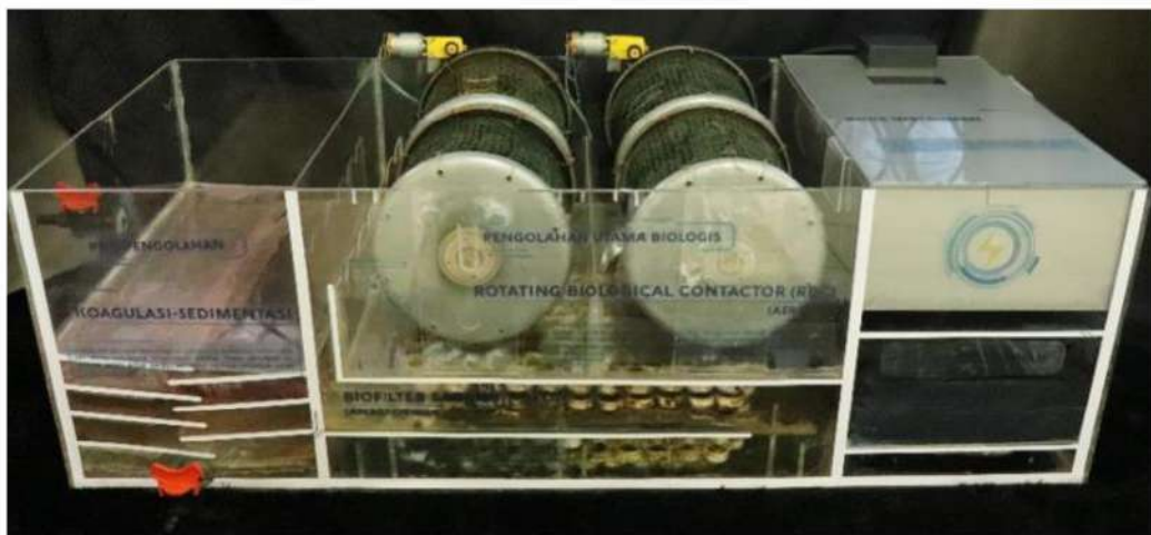
Gambar 1. Reaktor Pengolahan Limbah Cair Tekstil Berbasis Hybrid Attached Growth Biofilm Terintegrasi Arduino (Rahmadi et al. (2022).
